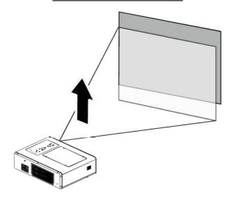
3. To alter the picture size, press Menu and select the Adjust menu using ▲or▼. Press ← to open the Adjust menu. Press ←or▶ to select Image Options followed by ▲or▼ to select Screen. Press ←.
